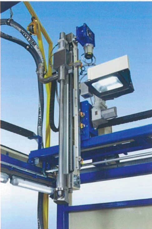
Built-In Camera System to address drum bunghole for filling operations.
